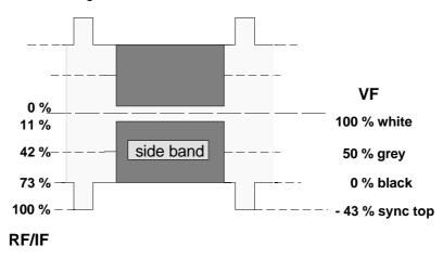
Level Percentages for RF/IF Signal with Reference to VF Signal
