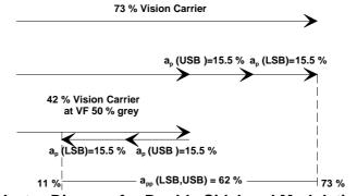
**Vector Diagram for Double Sideband Modulation**
